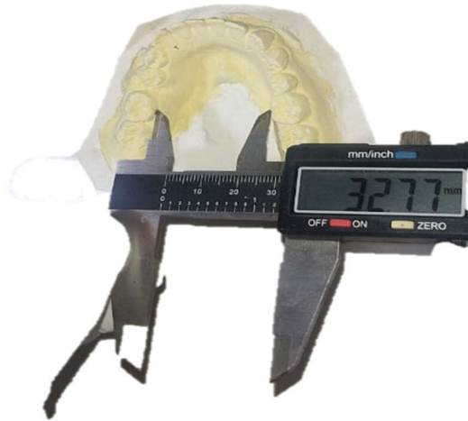
Figure 2: Measurement of IM width using a Digital Caliper (European Directive ROHS 2002/95/CE)
