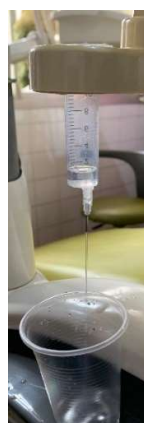
Figure 2: Simple capillary viscometer
